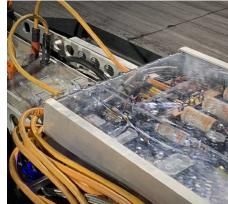
Isabellenhütte's IVT-S "smart shunt" supplies the data to balance battery life and raw power/torque.
