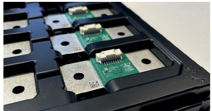
Fig. 2) Users no longer need to record the initial resistance value and the temperature curve (TCR) of each component, as this data is provided directly on a data matrix code.
