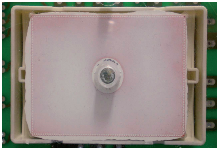
Figure 2: Excellent distribution of thermal grease is achieved. Experimental setup with glass plate
