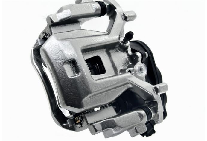
*With an EPB, the switch in the car's interior starts up the actuator, which presses the brake pads against the brake discs. The control unit is set up with a fixed current profile for the EPB's contact pressure, which monitors the shunt when the EPB is activated. Image: ©Shutterstock*
