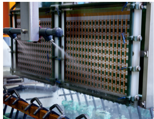
Plating process in new panel plating shop
