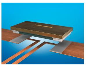
Image caption: An FMx shunt under construction: The resistance material, e.g. NOVENTIN®, is made of a robust full metal plate which is directly soldered with its underside. Very low-ohmic resistances are achievable thanks to the large cross-sectional areas.
