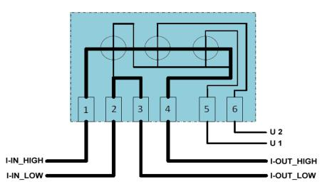
The I-IN LOW, I-OUT\_LOW, I-OUT HIGH connections I-IN HIGH, are made using M8 M8x35. The corresponding self-locking screws (4x) nuts are pre-assembled.
