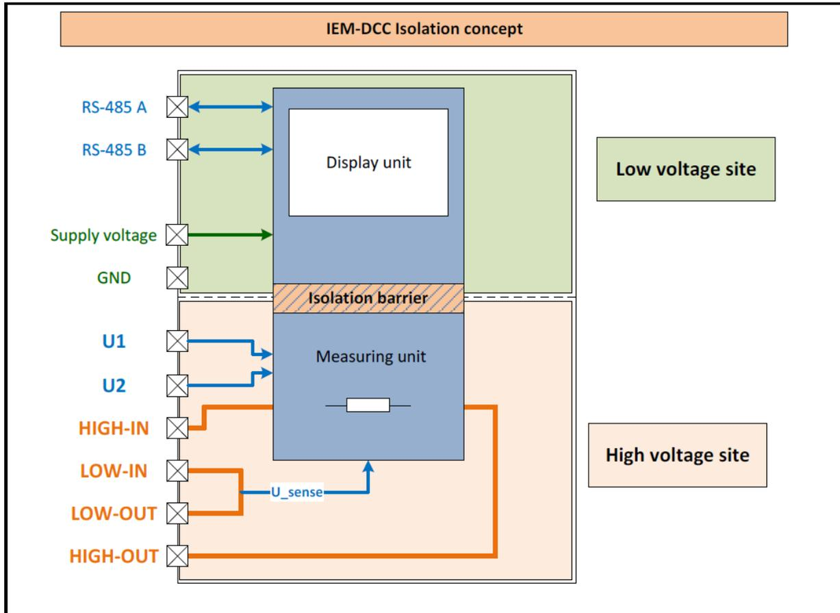
Figure 2: The IEM-DCC-500 features an isolated internal architecture. Source: Isabellenhütte
