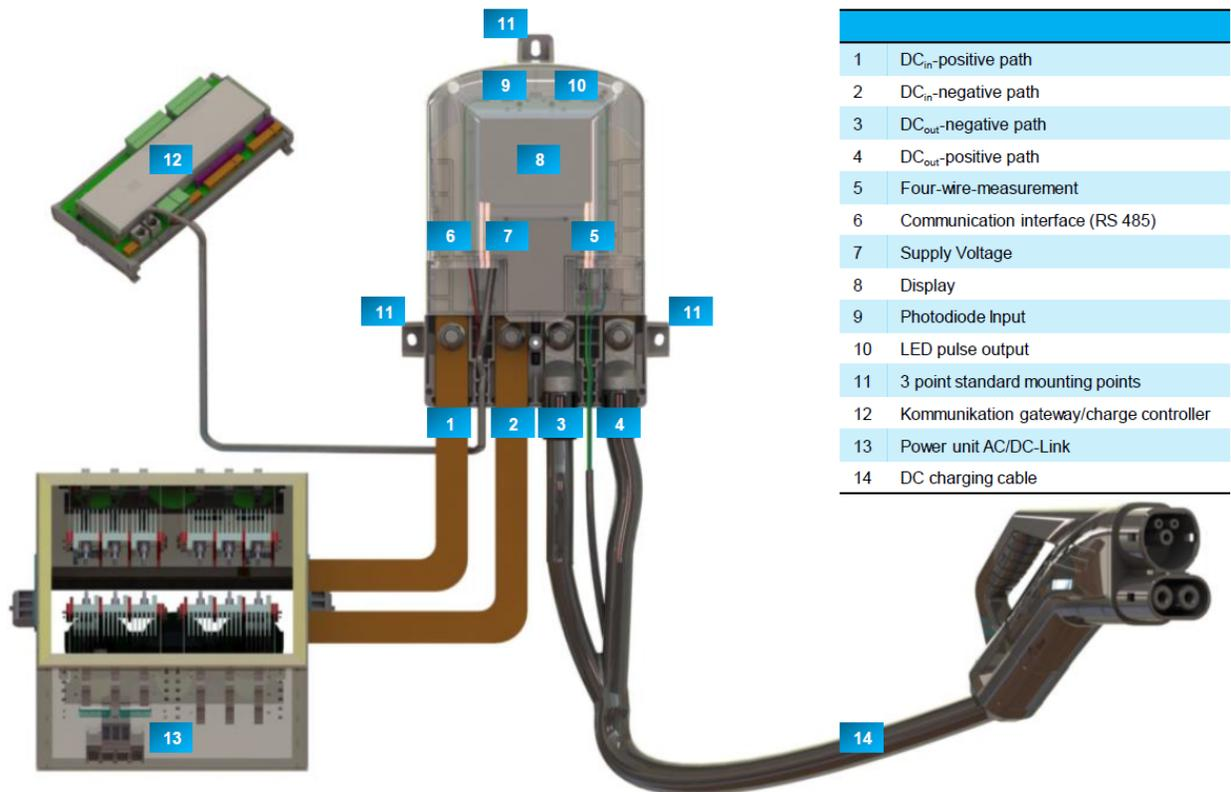
Figure 3: The DCC-500 energy meter provides a simple interface to the EVSE. Source: Isabellenhütte
